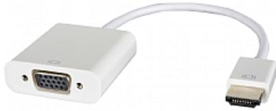
ADC-HM/GF is an HDMI™(M) to VGA(F) adapter cable. Short and flexible in design, this active cable converts a digital HDMI signal to an analog video signal while outputting the HDMI audio to a separate stereo audio output.
